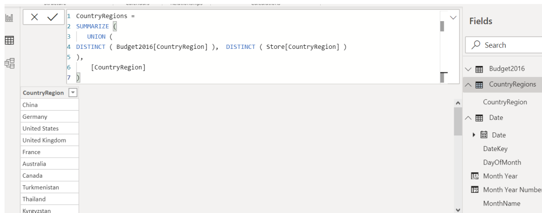
Figure 6-11: You can populate a calculated table with the distinct values of CountryRegion.
